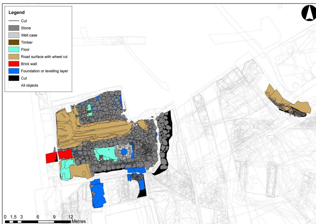
Fig. 195. The new gate building with revetments, road surfaces and bulwark. The expansion and reinforcement of the gate eastwards includes parts of the Late medieval moat and runs on an estimated north-south line about 2 metres east of the well. The void among the foundation stones is caused by modern shoring on the building site.
