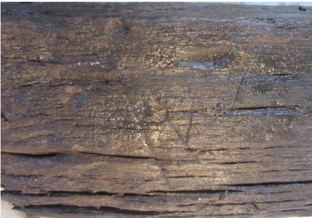
Fig. 64. A possible positioning mark ("lv") on timber (ST70895). From Melin 2013:12.
