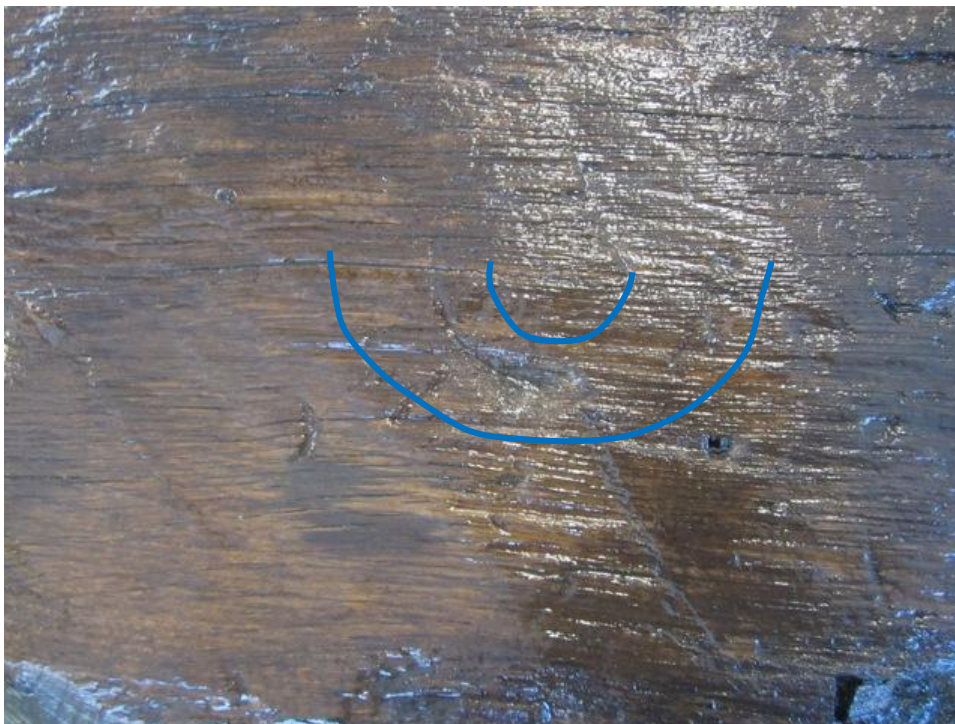
Fig. 65. Plank (ST70434) from SG-714 belonging to group B. The compass mark is visible in the middle of the blue lines. From Melin 2013:20.
