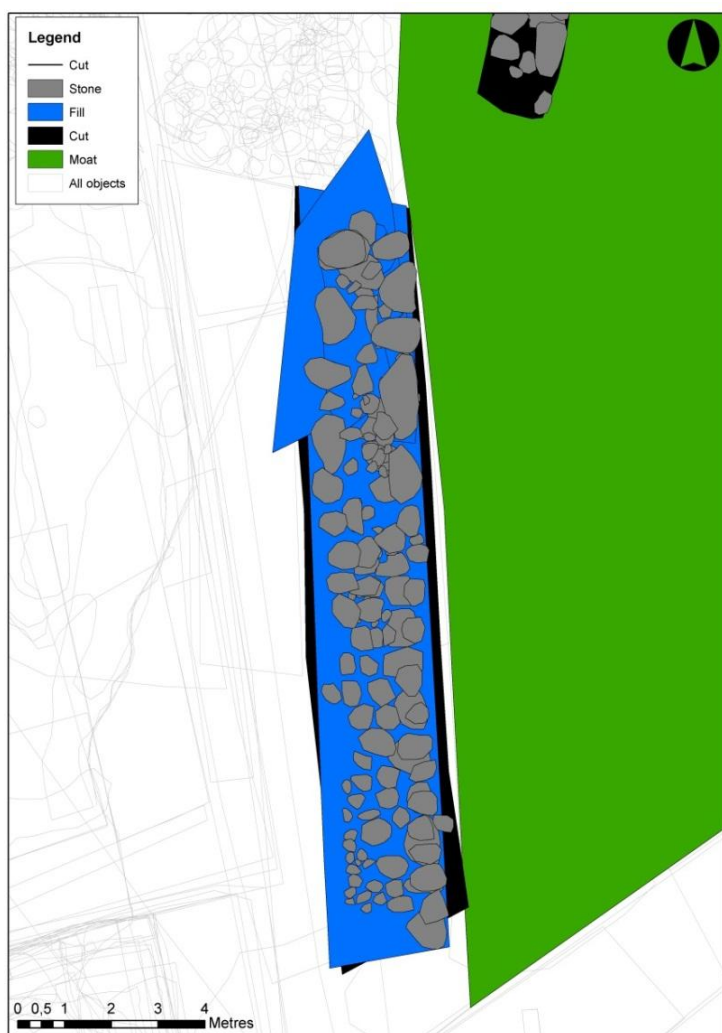
Fig. 163. North-south running curtain with construction cut, two courses of stones and boulders together with foundation layers. Part of the contemporary moat to the right.
