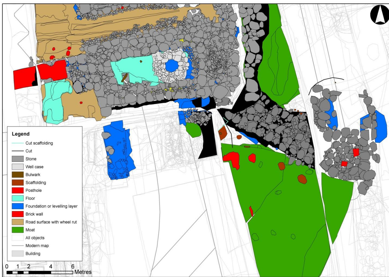
Fig. 182. Dam with semicircular barrier tower placed SW of the gate building in the Late medieval moat. The lack of stones in the middle and within the tower is due to the modern shoring and a concrete pillar erected in conjunction with the new Guide Wall. The measured moat cut to the left, inside the building should be moved two metres to the right based on later re-interpretations.
