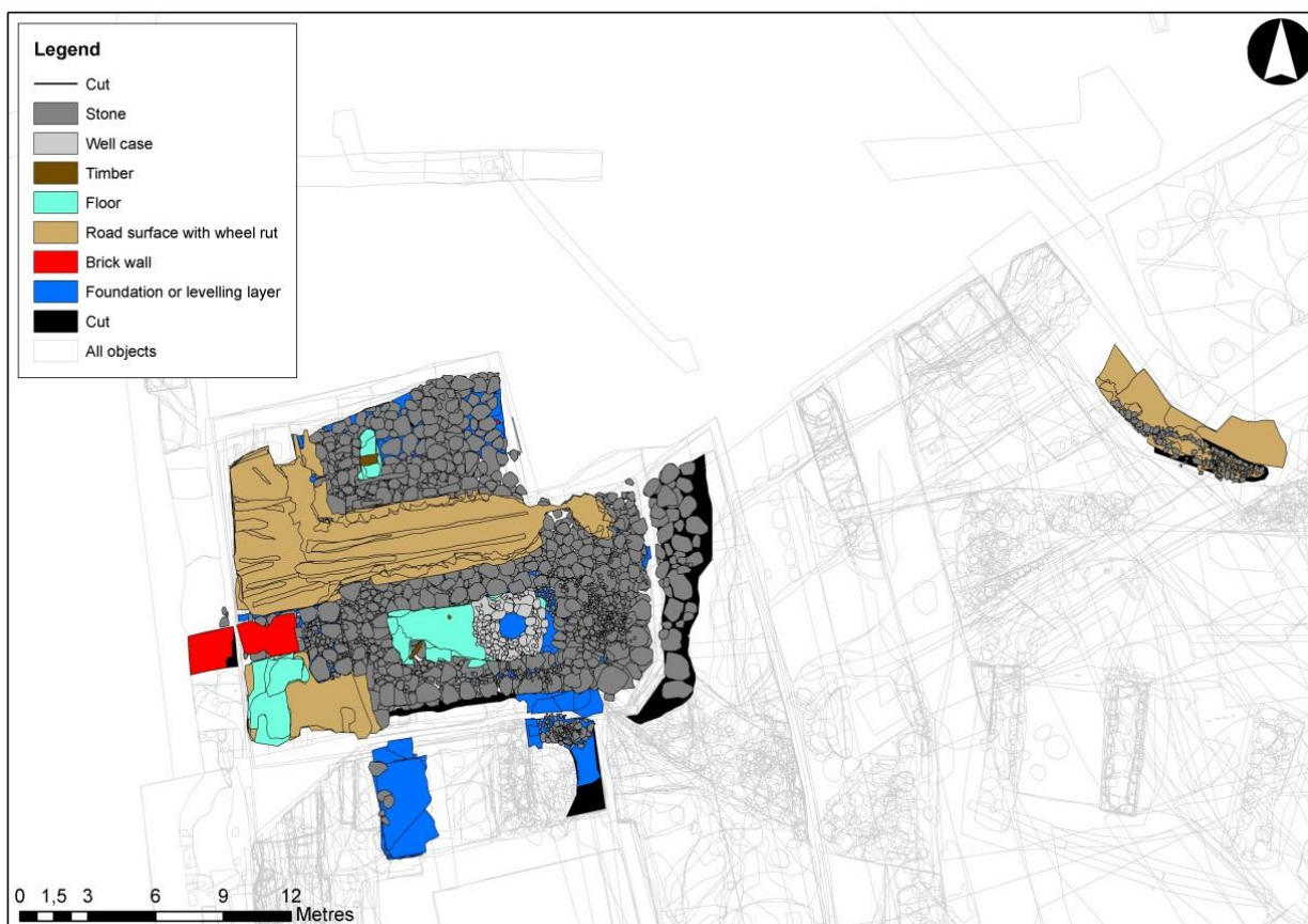
Fig. 144. The new gate building with revetments, road surfaces and bulwark. The expansion and reinforcement of the gate eastwards includes parts of the Late medieval moat and runs on an estimated north-south line about 2 metres east of the well. The void among the foundation stones is caused by modern shoring on the building site.
