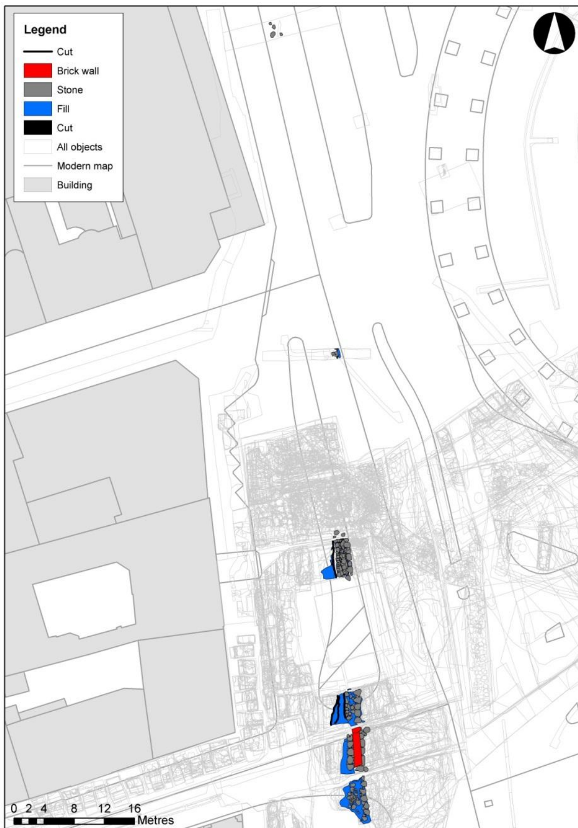
Fig. 62. Overview of investigated medieval city wall with construction cuts, foundation stones, limestone ashlar and brick walls outside Hotel D'Angleterre and between Lille Kongensgade and Østergade.
