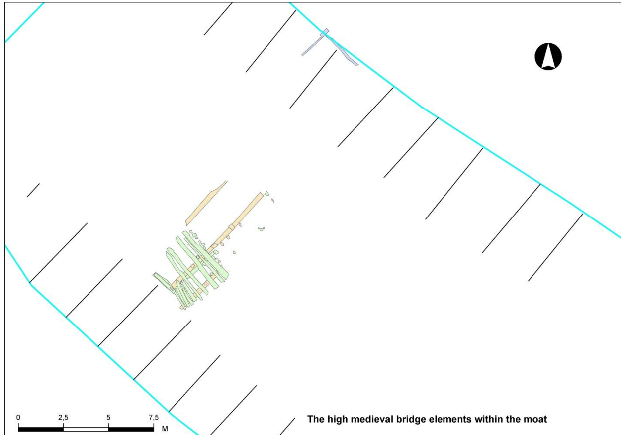
Figure 31 Plan of bridge elements, from c. A.D. 1372 (yellow and lilac) and later additions (green)
