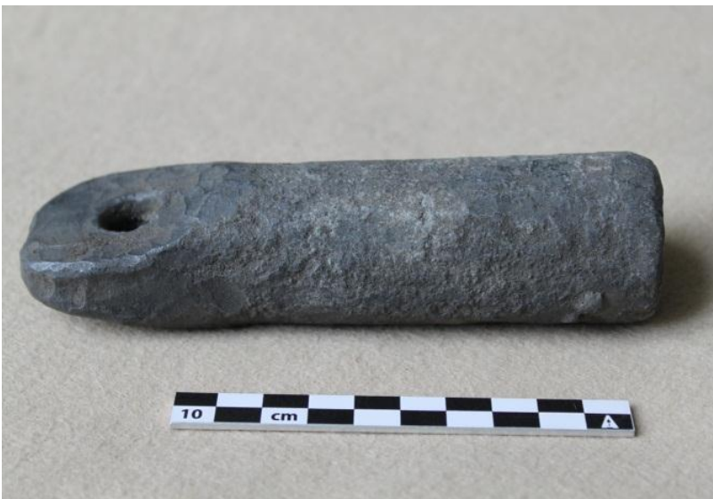
Fig. 130 FO 212461. A lead line to ascertain the depth of water. Recovered from SD53332 (G629)
