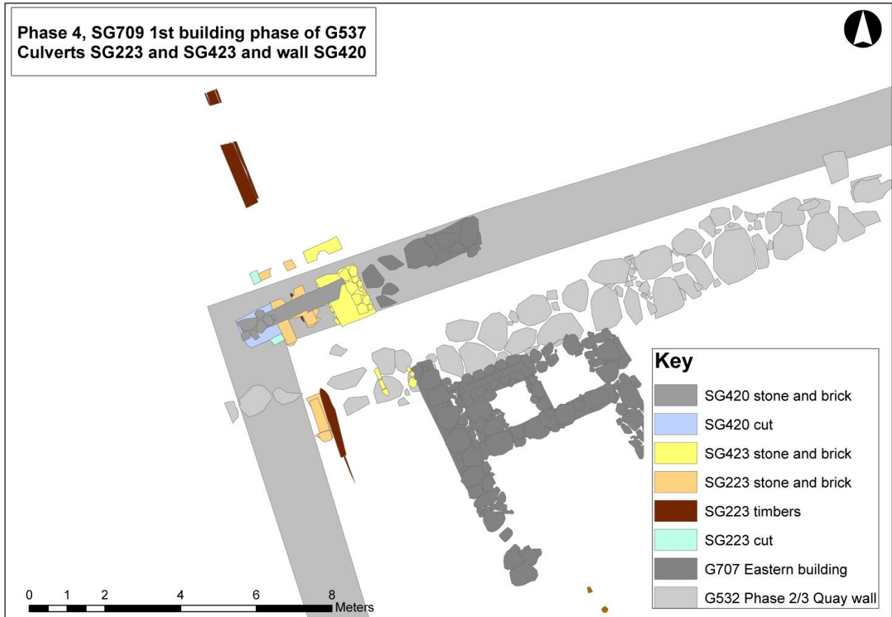
Fig. 257 Plan of the two brick arched culverts SG223 and SG423 with wall SG420 overlying
